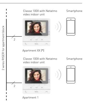
(\*) NOTE: for the sizing of multi-family systems refer to the General Installation Standards of the 2 Wires System Technical Guide.
